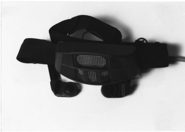
FIG. 2. Photograph of the head-mounted vision substitute sensors that radiate and receive the continuous transmission frequency modulated octave band ultrasonic waves. The small oval sensor radiates the waves for echolocation. The remaining three sensors act as receivers of the reflected and scattered waves from the object space.
