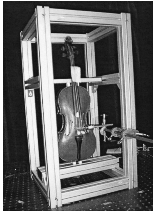
FIG. 5. The violin mounted in the measurement cage. The violin is squeezed between four rubber blocks at the top end and bottom end of the ribs, seen in the figure. The driving unit excites a small magnet glued to the treble side of the bridge. The cage made the measurements flexible and more reliable.
