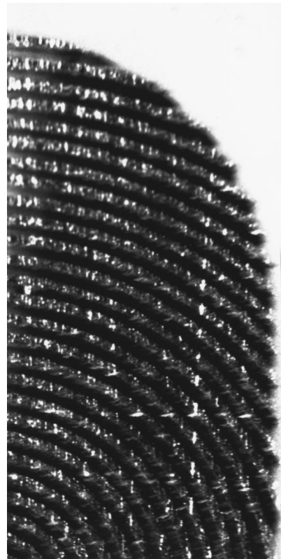
FIG. 3. A section of the backplate is shown of the large oval transducer seen in Fig. 2, showing the wide grooves and the treated rails that form the grooves.
